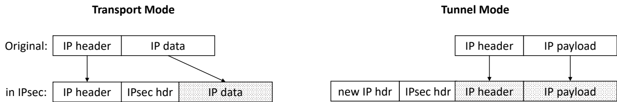
Figure 3: Comparison between IPsec transport mode and tunnel mode. All parts of the original packets that are shaded in gray are protected in the respective mode.
